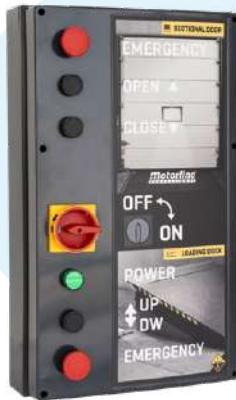
Electronic control board combined in a synchronized and safe way. Includes buttons to **open and close the gate**, button to **open/collect the dock leveler**, emergency and general cut-off buttons. This control board does not allow the dock leveler to be opened if the door is closed and, vice versa, it does not close the door if the dock leveler is open.
